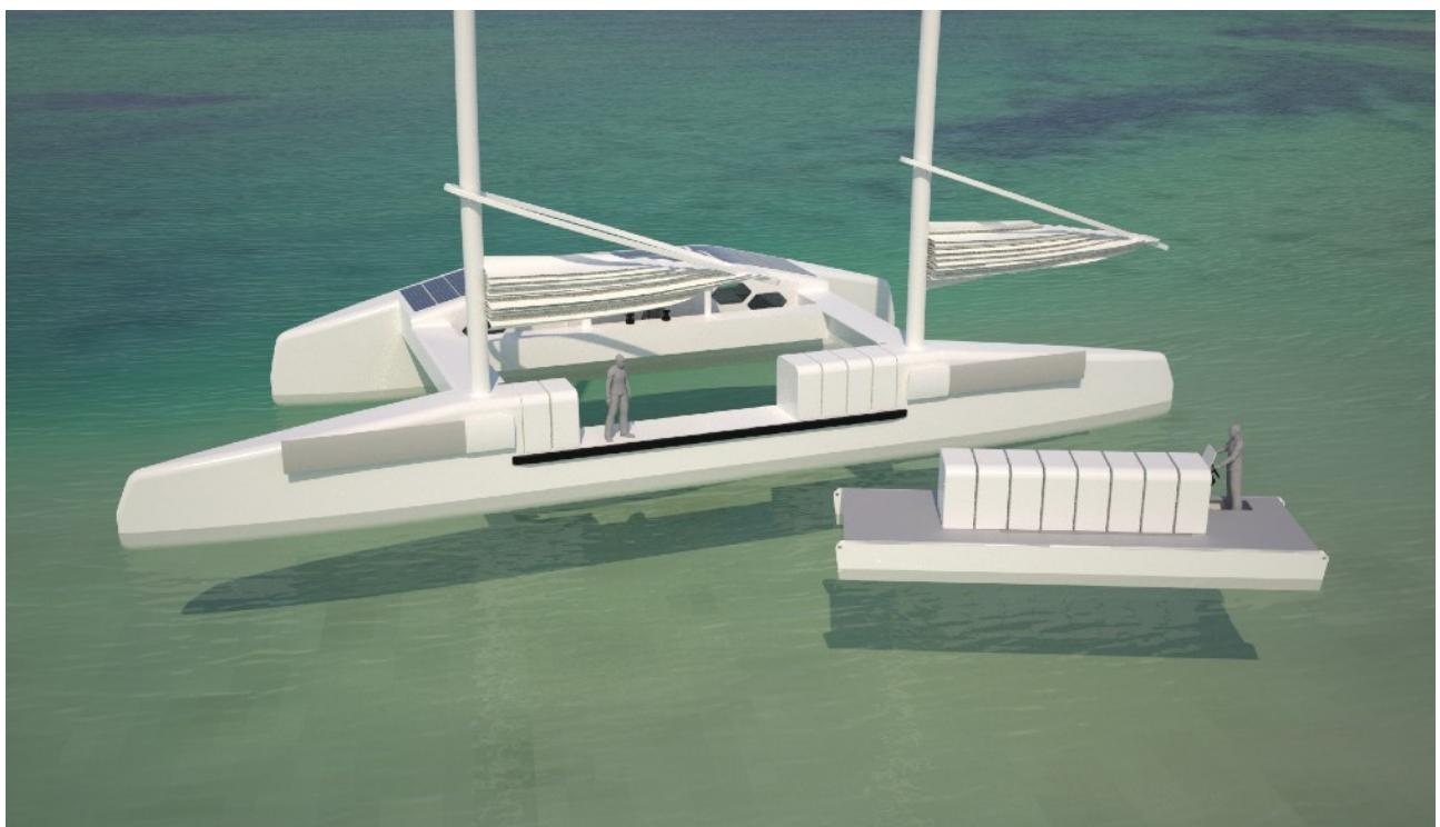
The tender bows are attached to the beam on the mothership with a hinge, allowing the tender stern to be lowered and the outboard used to power the mothership. This is the only source of external power for the mothership, which would be expected to sail anywhere as long as there was more than 6 knots of breeze. In less than this, the tender would propel it at ~6 knots.
