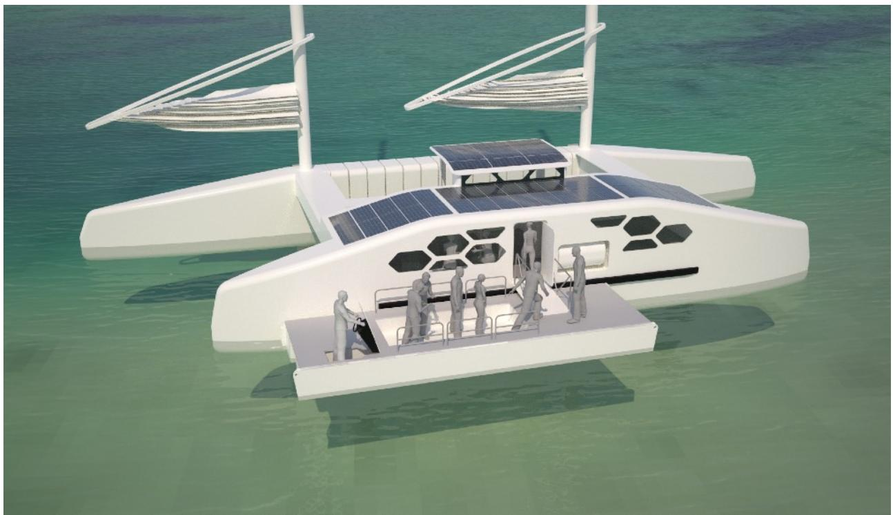
Access to the cabin is via a stairway on the windward side of the boat.
