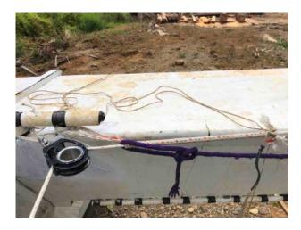
Made a crude textile clutch which works well for holding the top mast halyard, but may (will!) have some strength issues on bigger loads. I have some kevlar braid somewhere which will be much better.
