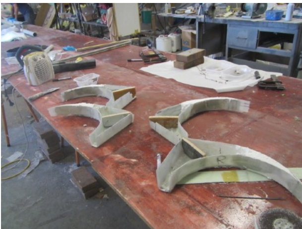
Beam to mast fillers
