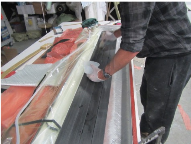
Carbon stacked and wet out
