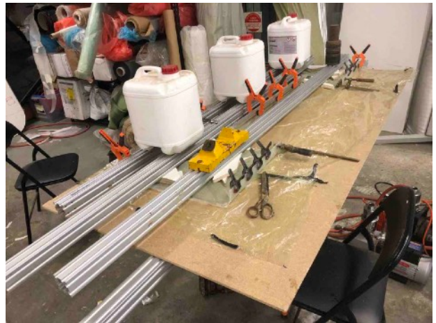
Gluing tender bulkheads together
