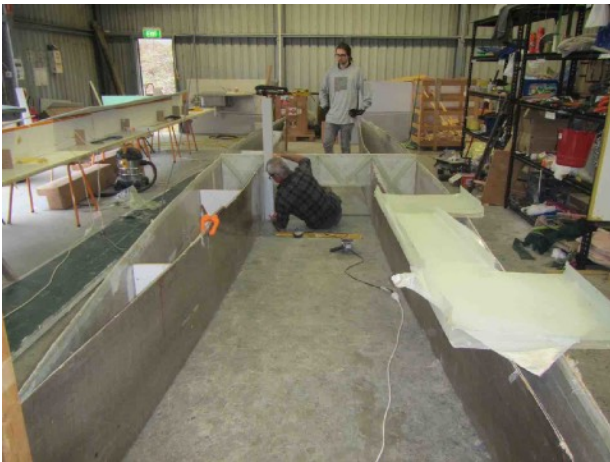
Fitting tender bulkhead
