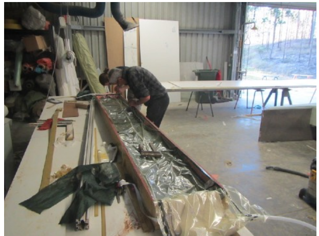
Leak sealing the bag
