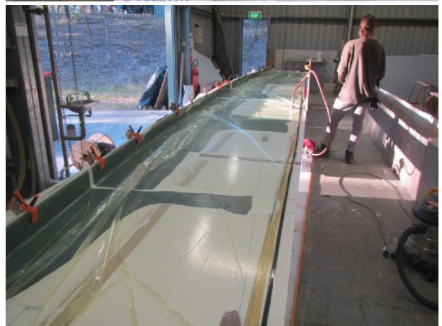
Fist deck half infusion. Pictures by R. Rasmussen
