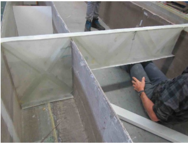
Fitting tender bulkhead
