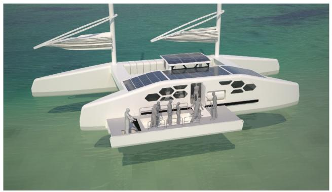
Access to the cabin is via a stairway on the windward side of the boat. Boarding is through an opening in the cabin side. The door can double as a gangplank if required.
