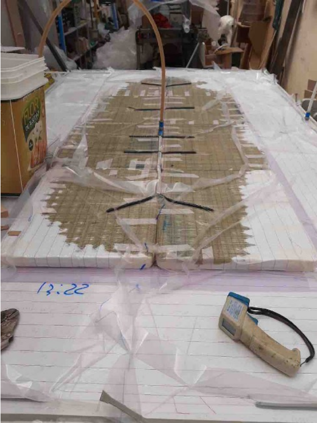
Beam bulkheads infusing
