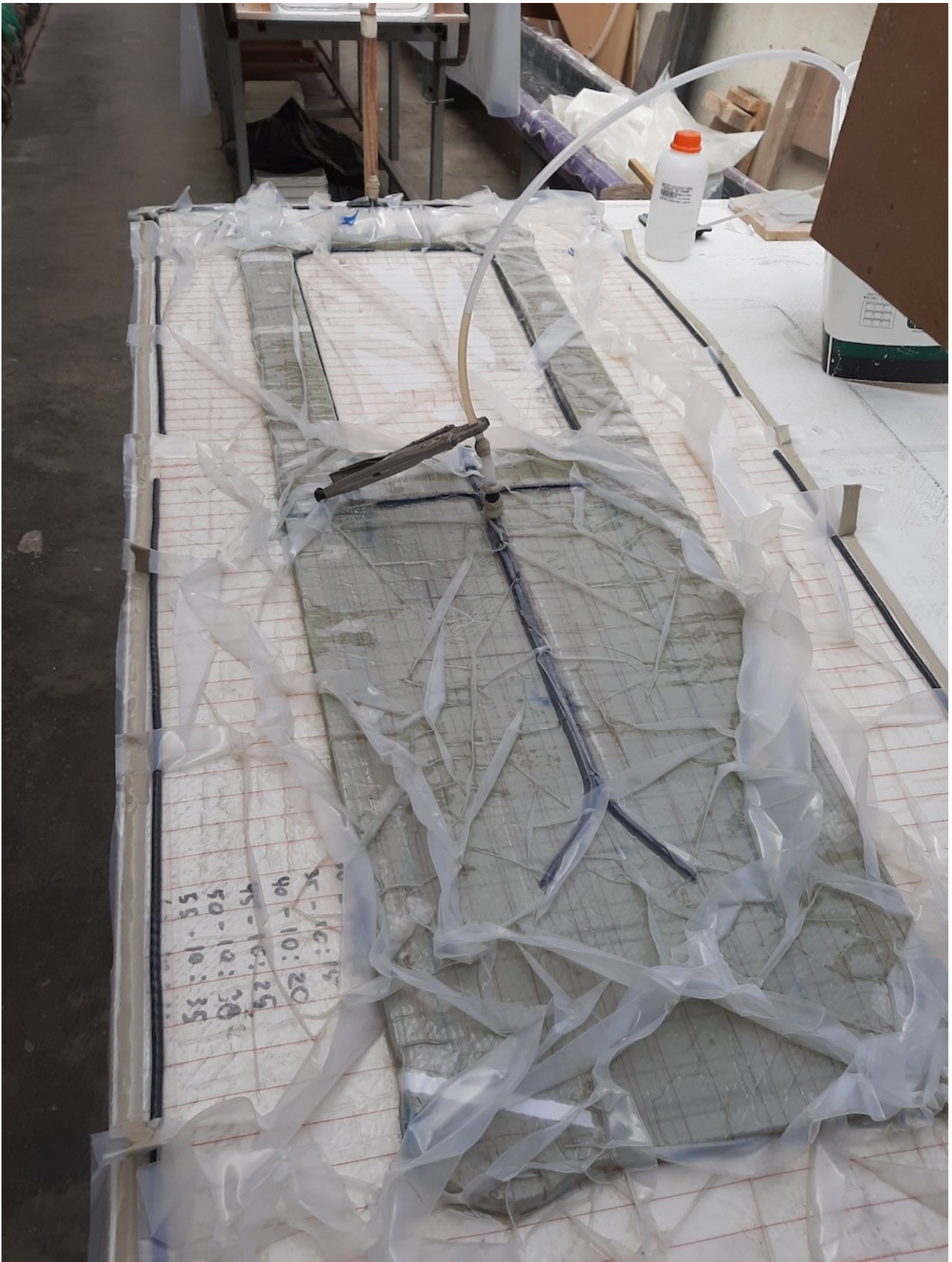
The optional bulkhead LW hull both ends. Made yesterday, (xmas infusion just for fun!). I decided to make it with an opening part, secured with watertight rubber seal and bolts. This will allow access to the area in case of necessity/repairs...
